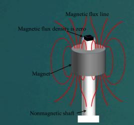
The magnetic field lines of the ringshaped permanent magnet enclosed in the head of the magnetic probe. The magnetic sensor is located at the magnetic null point at the top of the magnet. Tiny variations in the magnetic fields can be detected without the offset attributes from the nonzero magnetic fields. The amplifier gain can be enhanced optimally for tiny magnetic signals.
