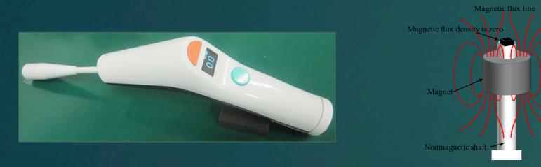
The magnetic field lines of the ringshaped permanent magnet enclosed in the head of the magnetic probe. The magnetic sensor is located at the magnetic null point at the top of the magnet. Tiny variations in the magnetic fields can be detected without the offset attributes from the nonzero magnetic fields. The amplifier gain can be enhanced optimally for tiny magnetic signals.
