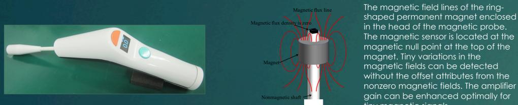
Fig. 1 Magnetic probe TAKUMI® (Matrix cell Research Institute Inc., Tokyo, Japan)
